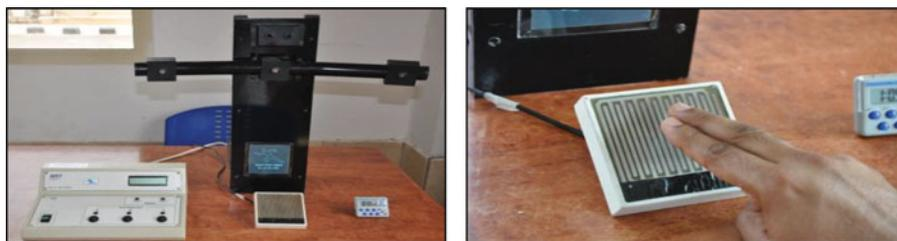
**Figure 2.** Measurement of reaction times. The reaction timer is shown to the left. The touch switch and resting finger position are to the right.
